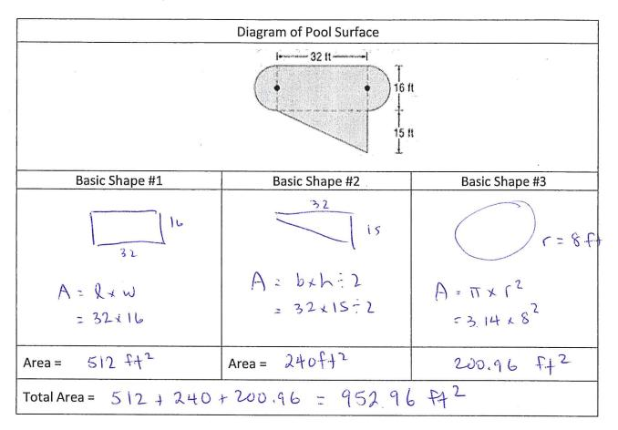
b) The pool is 6 feet deep. Use the formula:  $V_{prism} = Area \ of \ Base \times Height \ of \ Prism$  to find the volume of the entire pool.
